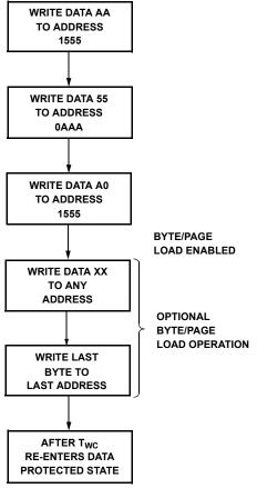
FIGURE 7. WRITE SEQUENCE FOR SOFTWARE DATA PROTECTION
