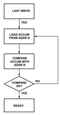
FIGURE 5. TOGGLE BIT SOFTWARE FLOW
