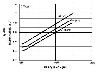
FIGURE 10. NORMALIZED I<sub>CC</sub>(RD) BY TEMPERATURE OVER FREQUENCY DATA PROTECTION
