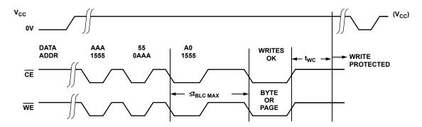
FIGURE 6. TIMING SEQUENCE—BYTE OR PAGE WRITE
