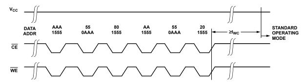
FIGURE 8. RESET SOFTWARE DATA PROTECTION TIMING SEQUENCE
